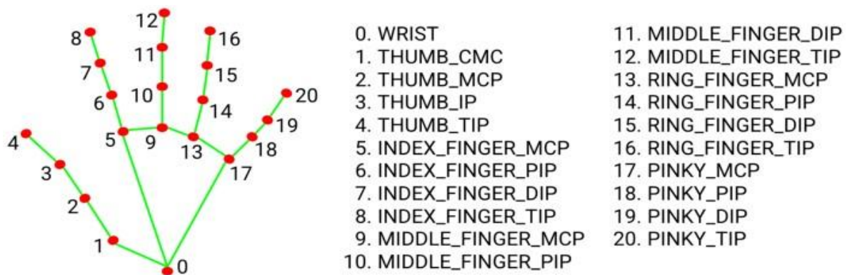
Figure 3: Mediapipe Algorithm hand coordinates
