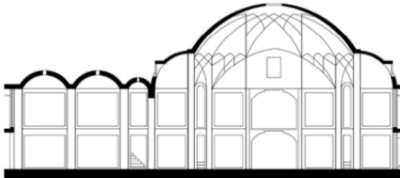
Figure 13: The Domes Are the Crossing Point Of Two Rasteh. (Shalchi, 2013)
