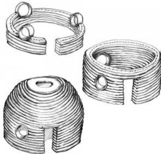
Figure 16: How to place windows in Adobe (Saeed Sun, 2012).
