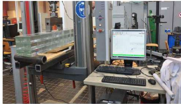
(b) Experimental set-up of the 4-point bending tests (Oikonomopoulou, Veer, Nijse, & Baardolf, 2015)
